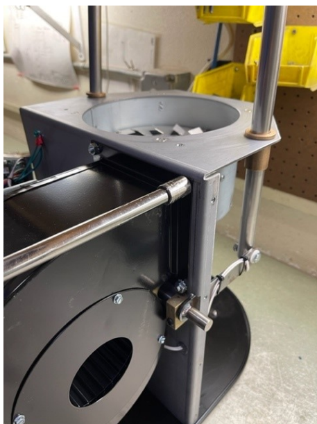
Remove mounting nuts with 7/16 socket wrench (4X)
